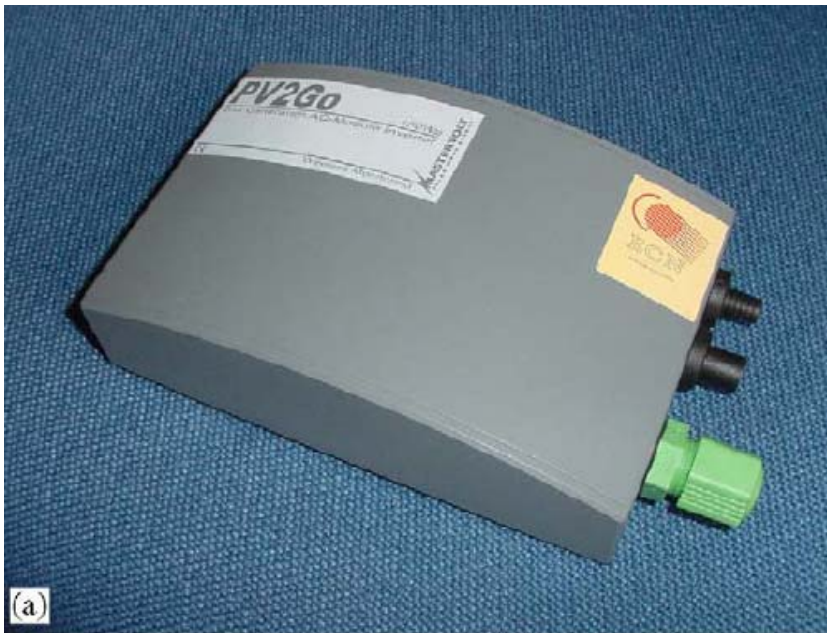
(a) The second prototype of the PV2GO inverter. (b) The second prototype of the PV2GO inverter without enclosure.
